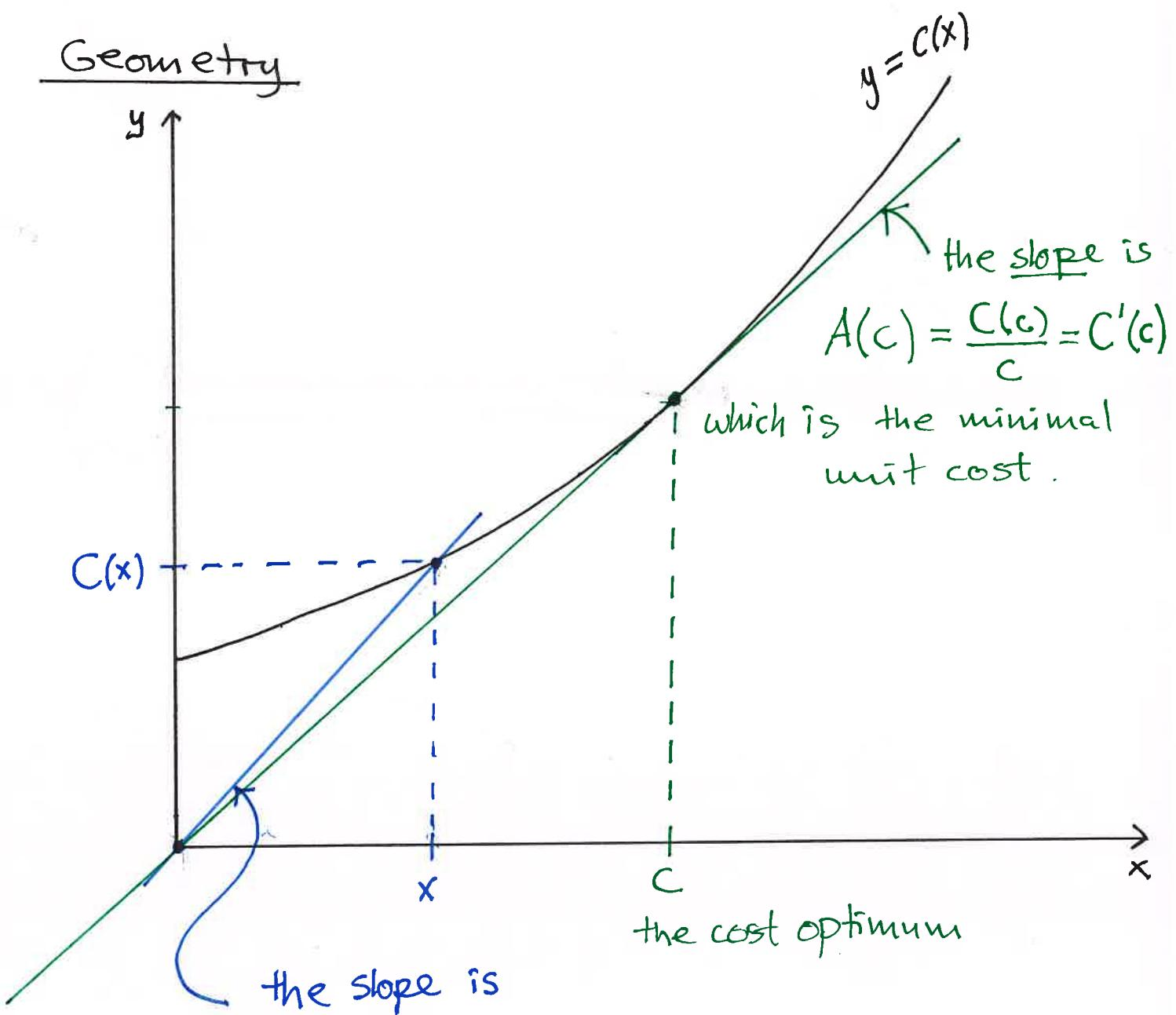
and  $A(c) = \frac{C(c)}{c}$  is the minimal average unit cost when  $C'(c) = A(c)$ .
